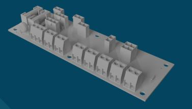
For AC type fans, speed control can be done with 0~230V voltage control. Therefore, the PWM output of the control card needs to be converted at 0~230V.
